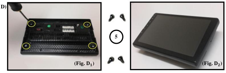
**D**) The 9 Inch radio must be screwed to the upper frame with the screws provided in the kit (5) (**Fig. D**<sub>1</sub>) creating a single body (**Fig. D**<sub>2</sub>).
