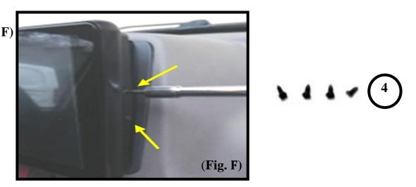
**F**) Both locking pins will be secured to the entire structure, using the 4 black screws supplied in the kit (**Fig. F**).
