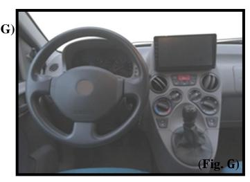
**G**) This is one of the possible solutions (**Fig. G**). The kit can be used on various models of 2DIN radio faceplates that comply with the internal dimensions of 183 mm x 105 mm.
