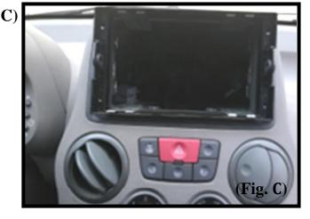
C) Install the assembled parts (faceplate + lower frame) in the vehicle (Fig. C).
