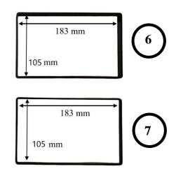
**A)** Position the lower frame (2) inside the radio faceplate 2DIN, if necessary using one or both of the adapter frames supplied in the kit (6 and 7).
