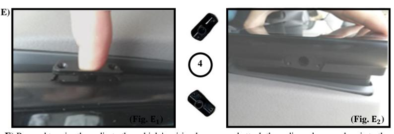
E) Proceed to wire the radio to the vehicle's wiring harness and attach the radio and upper chassis to the lower chassis previously mounted on the vehicle with the faceplate.
