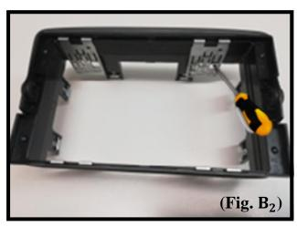
**B**) Place the lower frame at the correct height on the template 2DIN and proceed to assemble the parts, placing the metal brackets (3) at the 4 corners of the template 2DIN and clamping them to the outer edge of the template 2DIN using the tools to bend the fins of the brackets (**Fig. B<sub>1</sub>** e **Fig. B<sub>2</sub>**).
